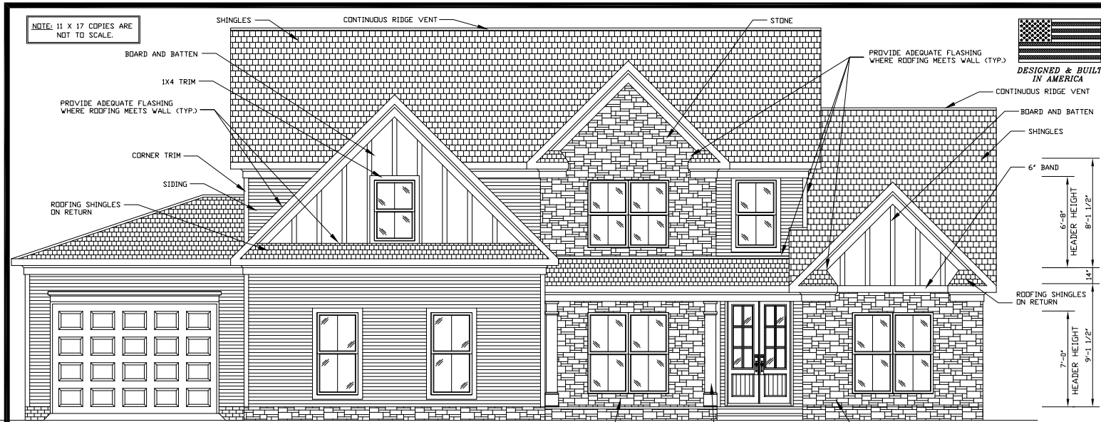
FRONT ELEVATION SCALE: 1/4" = 1' 0"
